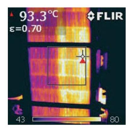
Uneven distribution of flow through plate heat exchangers
